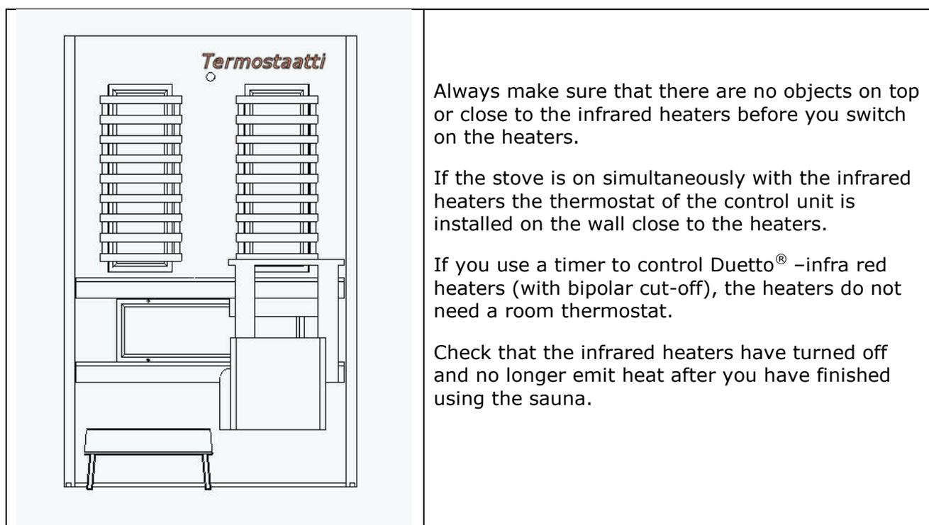
Always make sure that there are no objects on top or close to the infrared heaters before you switch on the heaters.
