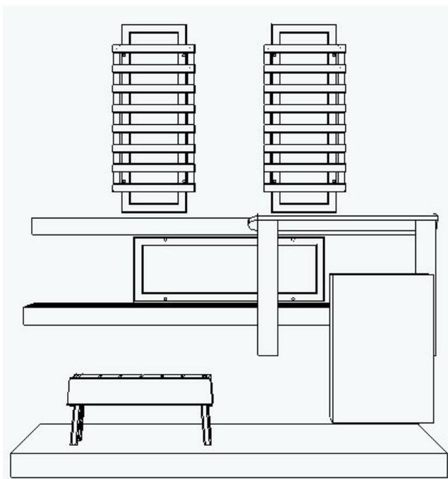
In a stove-heated sauna, the distance between a heater and sauna ceiling should be no less than 100 mm.
