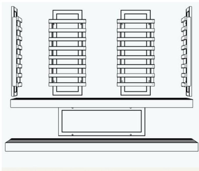
When the sauna size is about 4m<sup>3</sup> and you want to heat it up with Duetto® -infrared heater alone, five heaters is enough.
